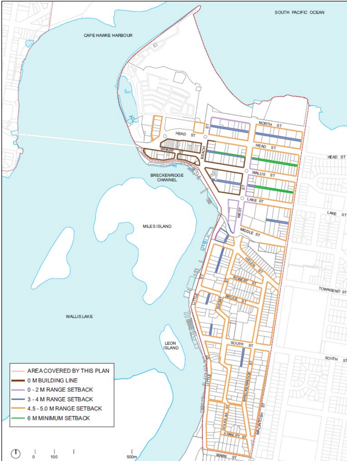
Forster town centre street alignment and setback plan (click here to view original image )
