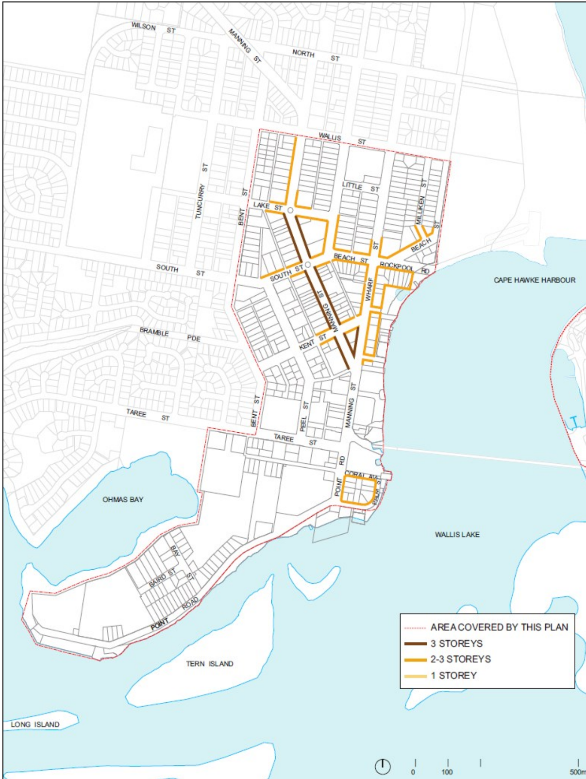
Tuncurry town centre street frontage height plan (click here to view original image )
