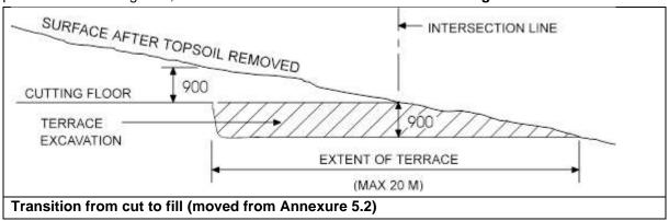
Extent of terrace: Extend the cut to the point where the cutting floor is 900 mm below the original stripped surface, or a distance of 20 m, whichever is the lesser.
