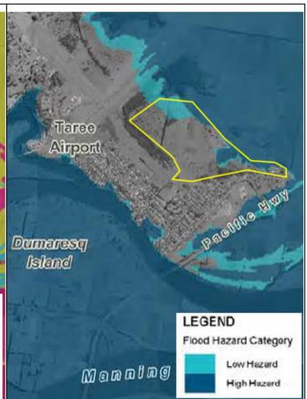
Manning Valley Flood Study 2016 1% AEP+2100 SLR true Flood Hazard
