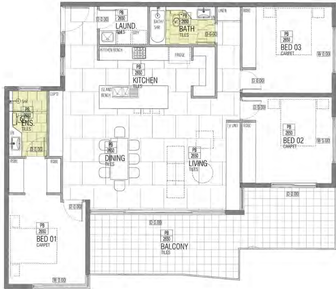
01 PROPOSED 3 BED - TYPE 01 1:50 @ A1 INTERNAL FLOOR AREA - 100.7m 2 EXTERNAL FLOOR AREA - 28.6m 2 GROUND - ROOM 1.10, 1.11 LEVEL 01 - ROOM 2.11, 2.12
