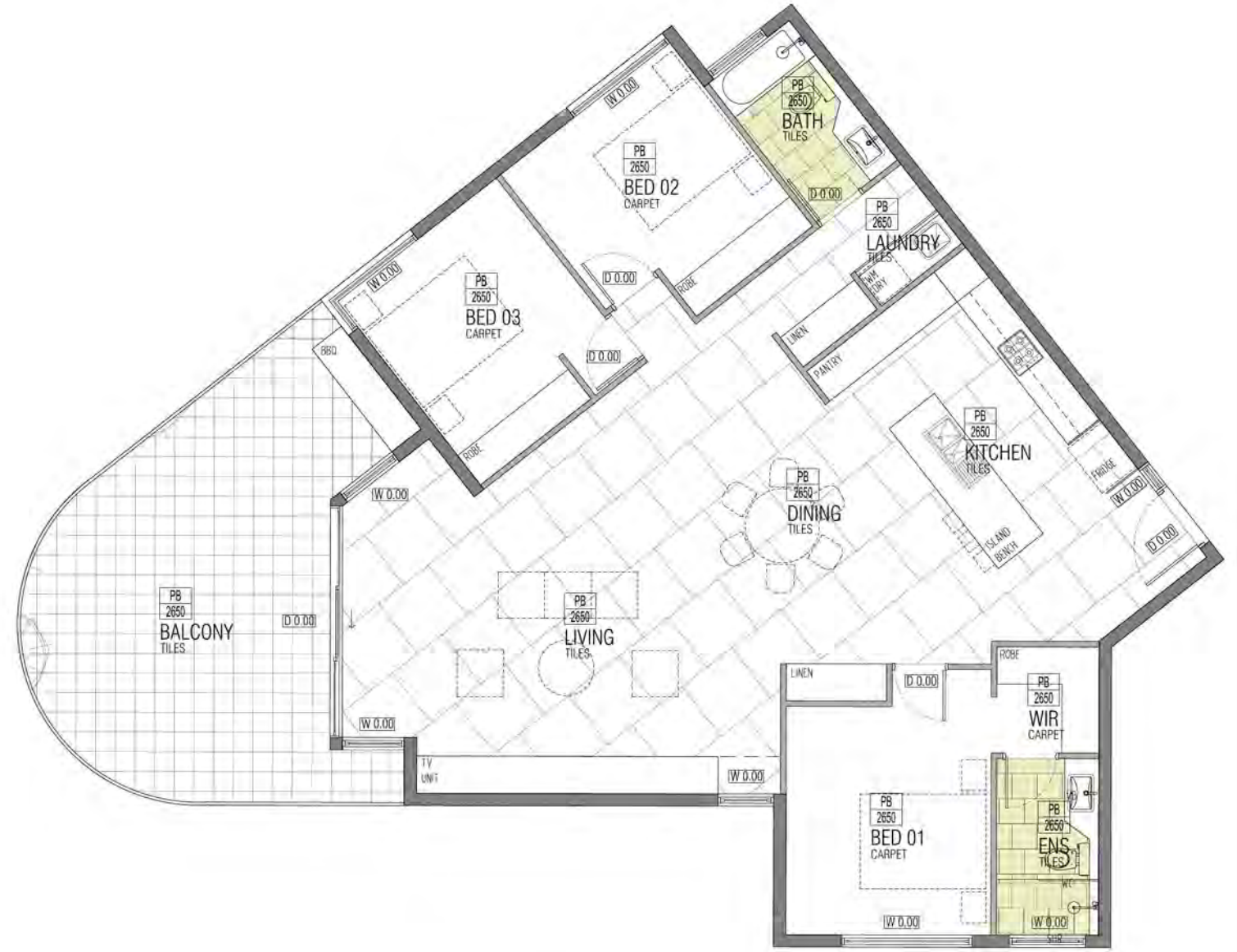
04 PROPOSED 3 BED - TYPE 04 1:50 @ A1 INTERNAL FLOOR AREA - 113.6m 2 EXTERNAL FLOOR AREA - 37.6m 2 GROUND - ROOM 1.01 LEVEL 01 - ROOM 2.01
