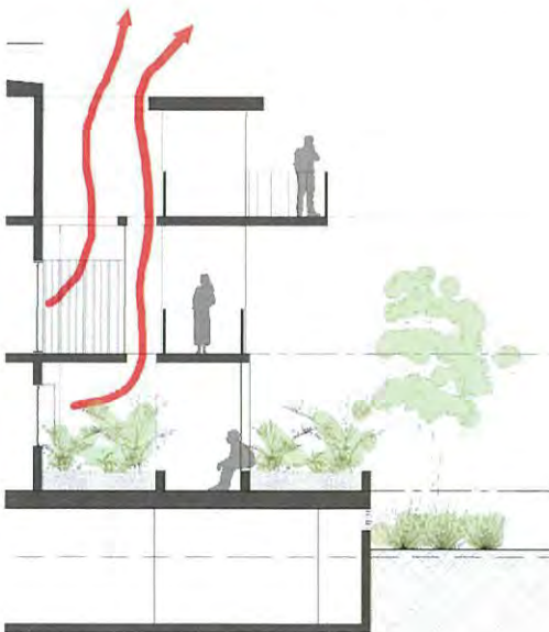
Image 11 – Ventilation: void space hot air expulsion
