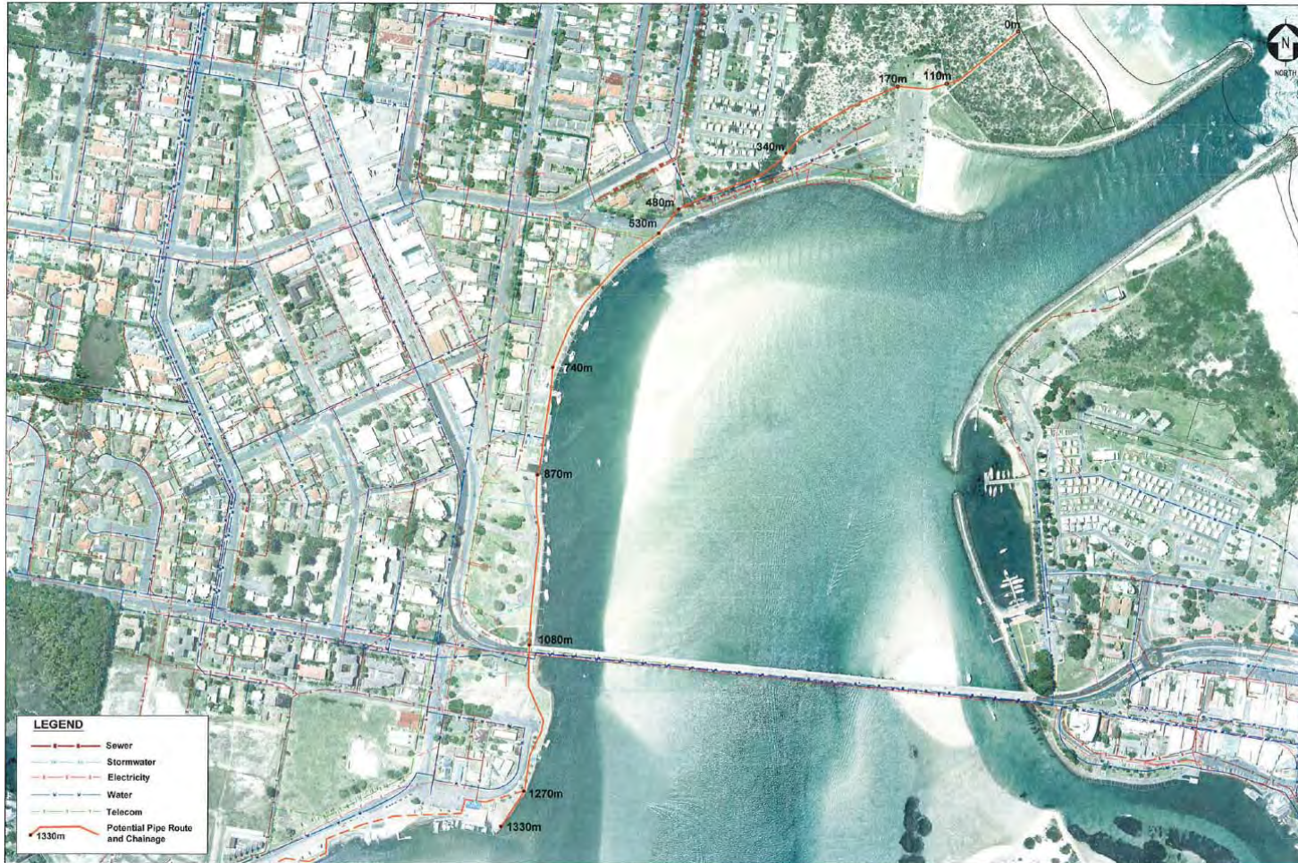
Figure 5.1 Potential Pipeline Route – Entrance to Boatland Marine
