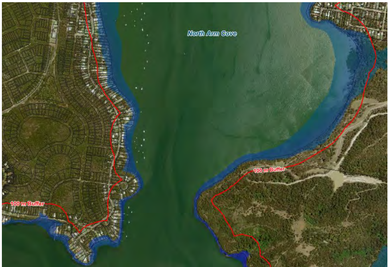
Figure 4-3 Adopted Mapping Methodology of 1% AEP Event; including Wave Runup level. Applied within 100 m of the Shoreline (indicated by Red Line).
