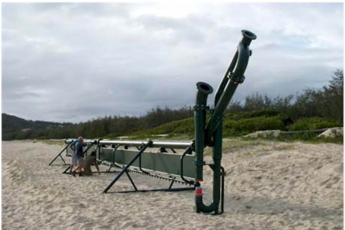
Figure 5-1 Sand shifter Permanent Sand Pumping System (source: Slurry Systems Marine)
