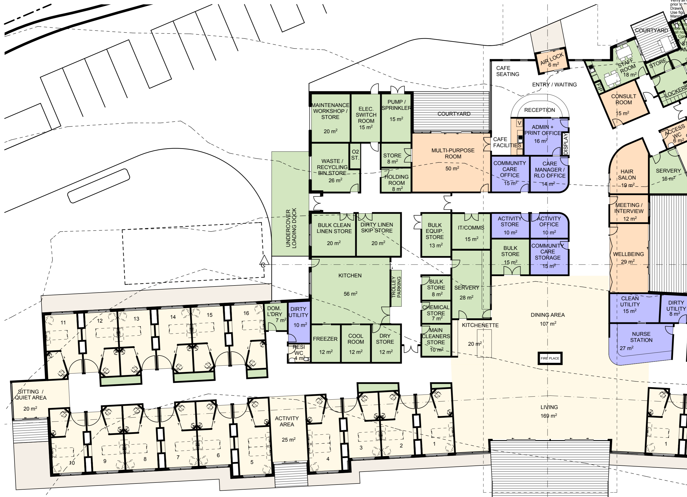
RACF Floor Plan SCALE 1:200 @ A3
