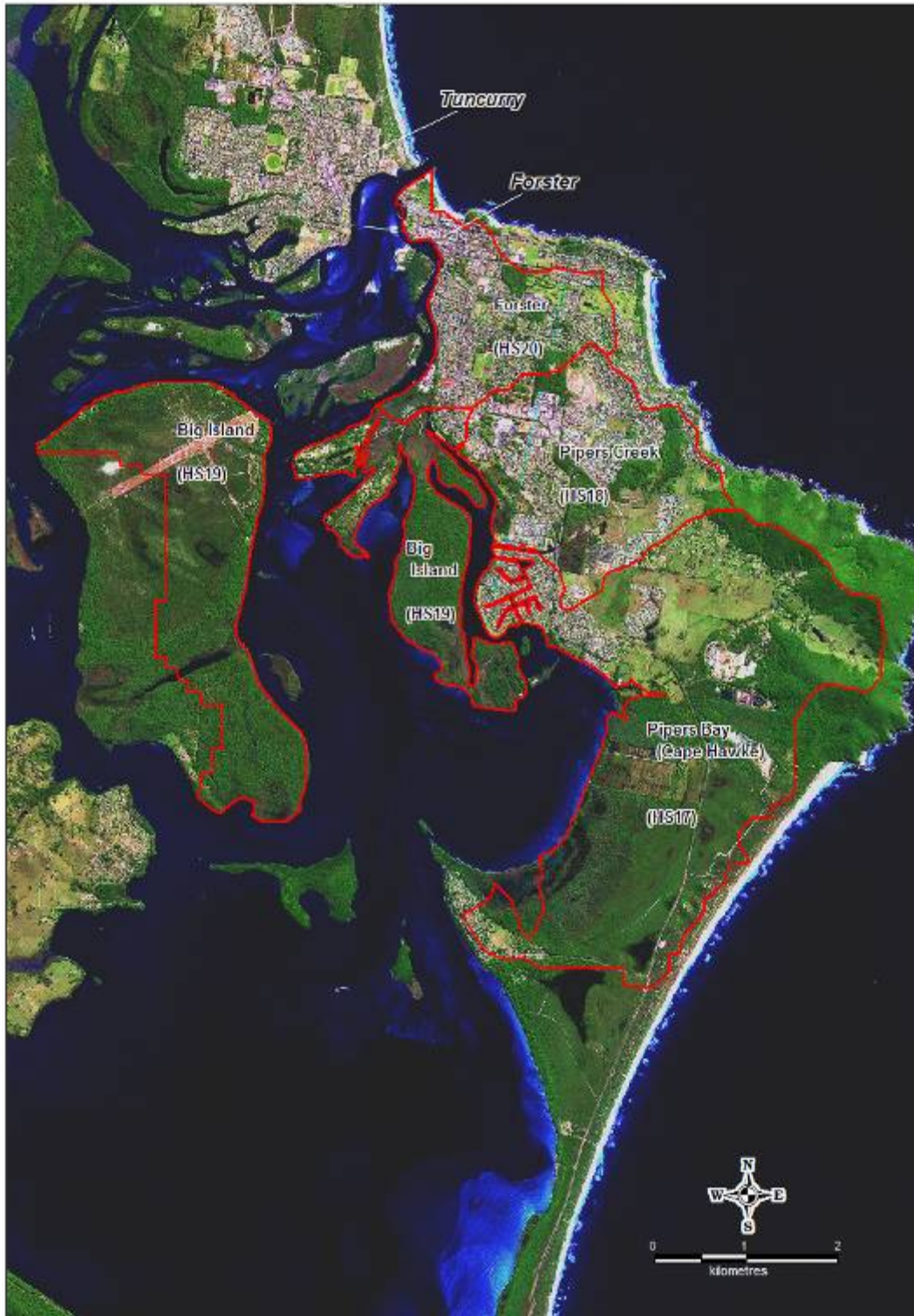
Figure 2.5.9. Forster sub-catchments draining into Wallis Lake. Pipers Creek and Bay are the receiving waters for sub-catchments HS17, HS18 and part of HS19.
