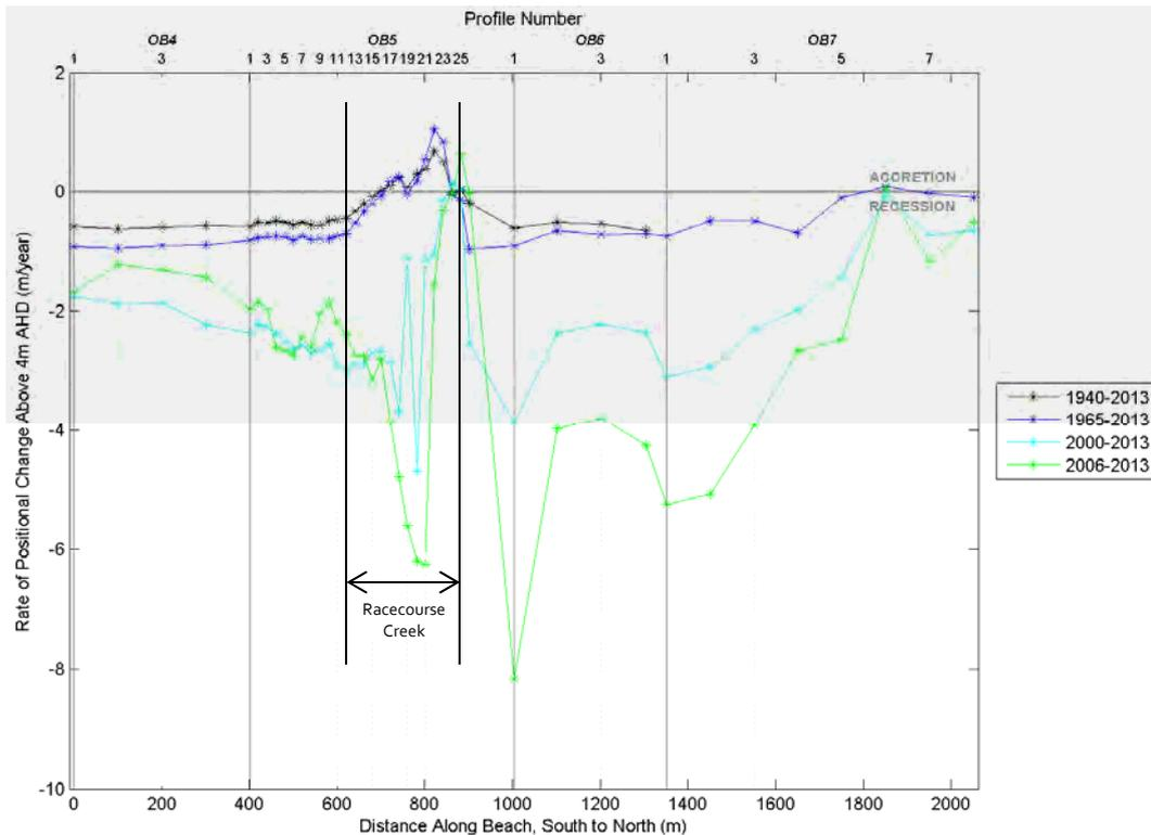
Figure E3 – Rate of positional change at RL 4 at Old Bar Beach
