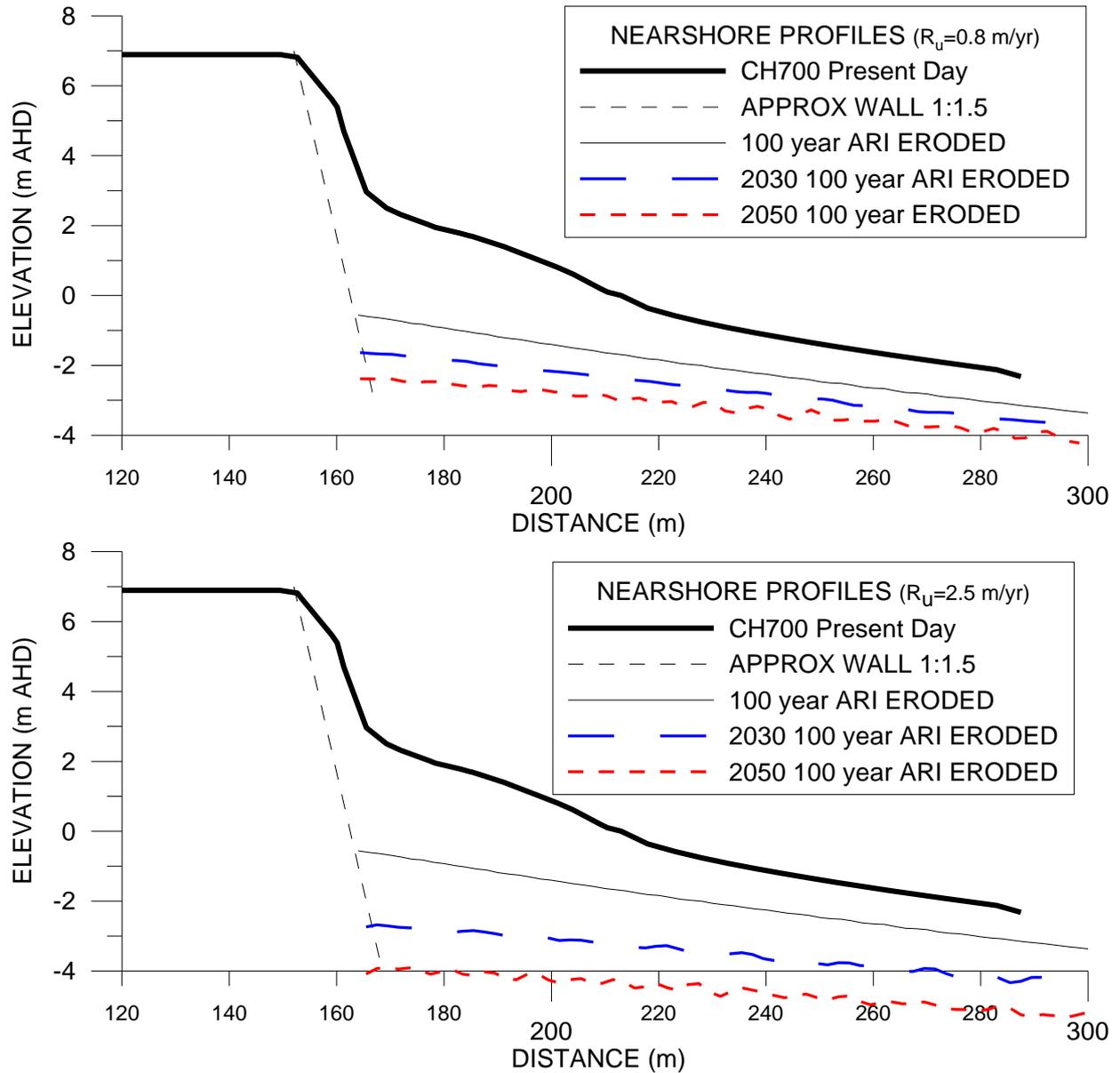
**Figure 3: Initial and Eroded Profiles at Seawall using SBEACH for Present Day and Future Planning Scenarios (using 0.8 and 2.5 m/yr Underlying Recession)**
