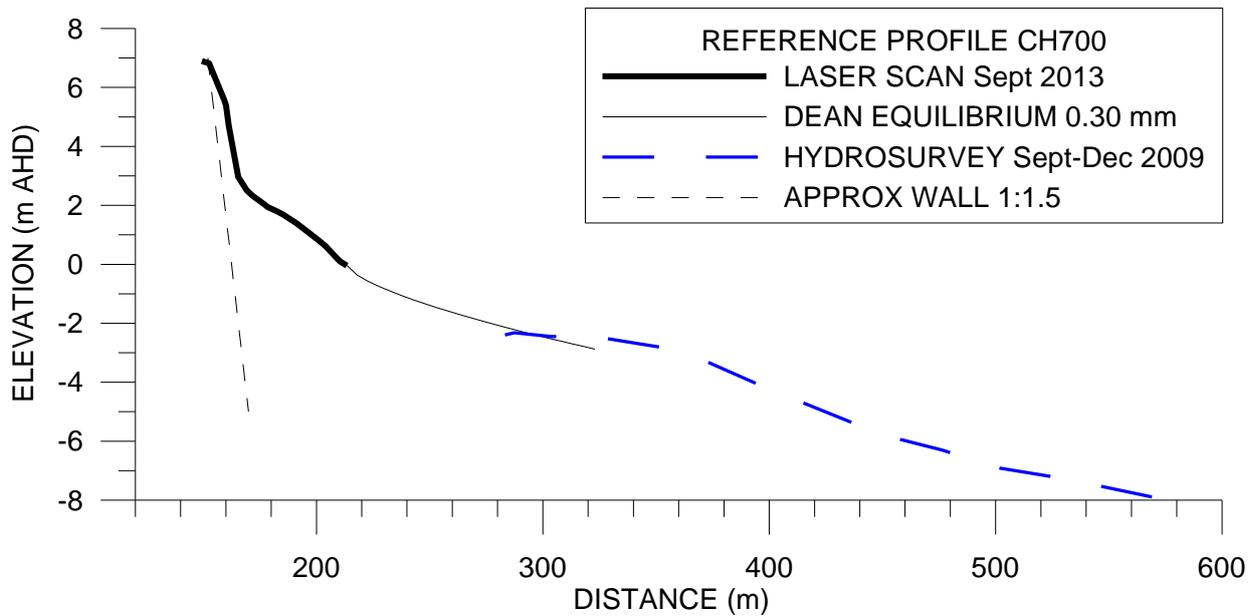
**Figure 2: Chainage 700 m Reference Profile based on 2013 and 2009 Data (source RHDHV)**
