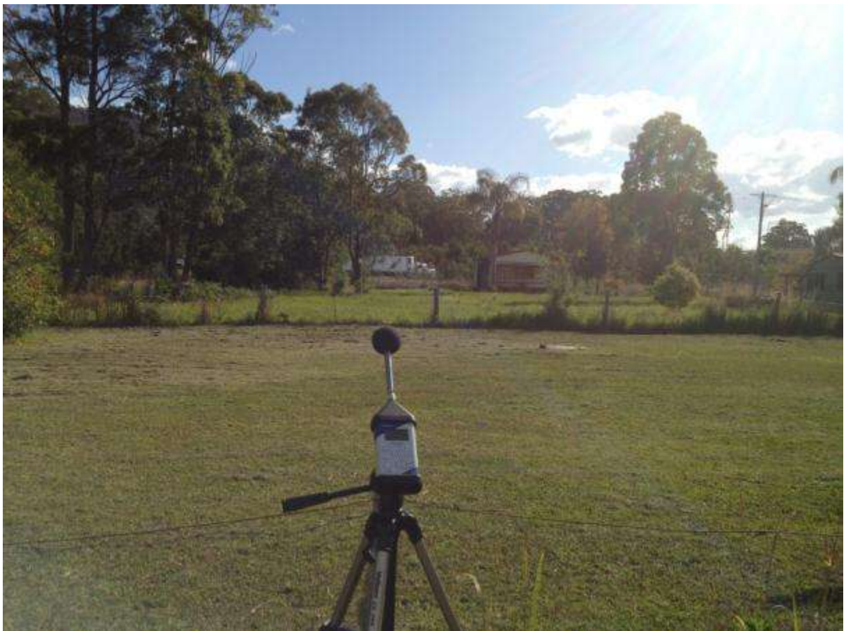
Photo 2: The SLM recording background noise levels on the boundary. The white truck is travelling on the Highway.
