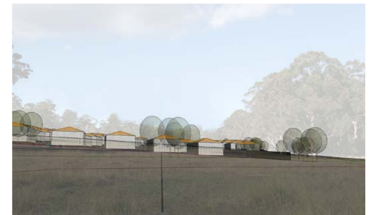
FIGURE 12.0. Perspective view is captured at precise viewpoint location in the 3D model then overlaid on the photographic image. Transparency settings are used to accurately place the model based on site boundaries and topography.
