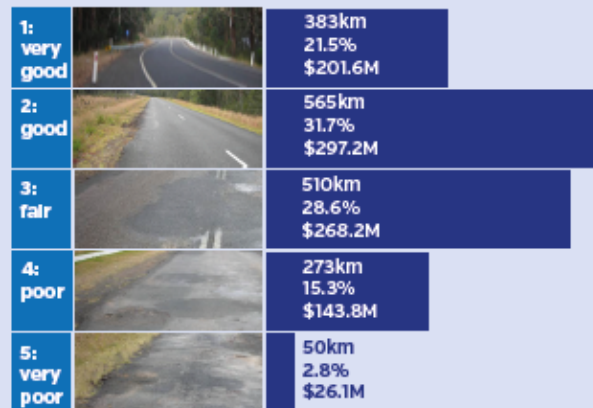
Around half of our 3,500km of roads are sealed. The graph above shows the proportion of our sealed road network by condition, indicating the length (km), percentage of total network, and value of roads in the current condition ($M).
